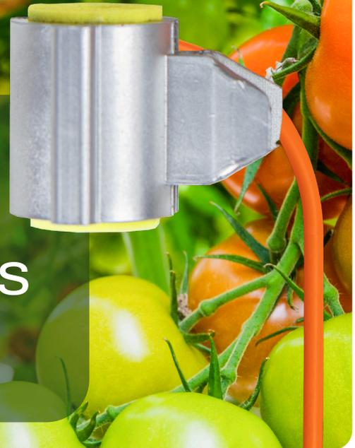
The Sap Flow sensor is designed for monitoring relative variations of sap flow rate in plants petiole or small shoot.
