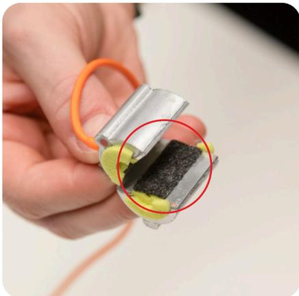
**Recommendation:** To securely position the sensor on stems with a diameter below 8 mm (approximately 0.31 inches), insert a foam-rubber bar into the internal cavity of the sensor, as shown below.
