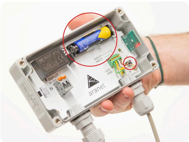
5. Insert battery and click the "PAIRING" button on the transmitter (left corner).
