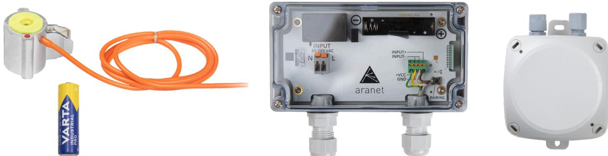
It is important to note that the sensor is already connected to the signal conditioner and transmitter, so all you need to do is plug in the power cable. But first, let's pair the Sap Flow sensor to the base station.
