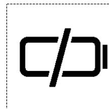
The battery is exhausted. Replace the batteries.
